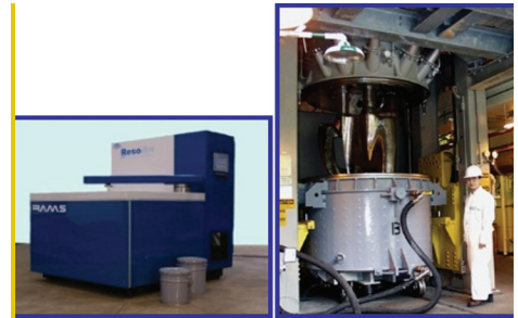
RAM-5 and existing production mixer
