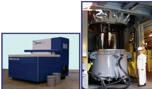
RAM-5 and existing production mixer
