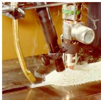
inputs can be used to compensate for low preheat (60oF), resulting in a favorable cooling rate for avoiding hydrogen cracking with current filler metals.
