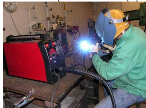
The prototype EB-200MP during testing at Electric Boat's welding laboratory.
