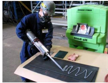
Apply Adhesive Hazardous Materials – Messy
