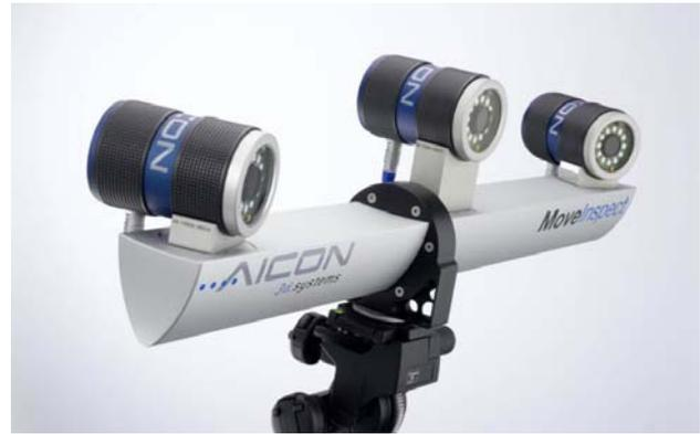
Trade friendly system will provide digital readout locations within a grid system on curved and planar surfaces
