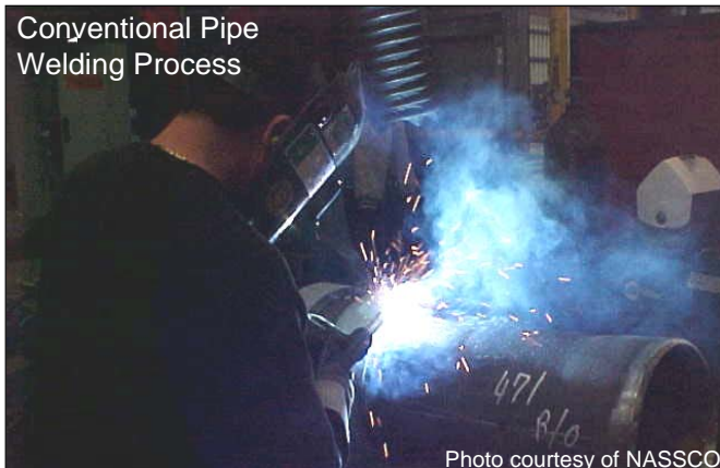
Figure 8. Photograph of the conventional pipe welding process (courtesy GD NASSCO).
