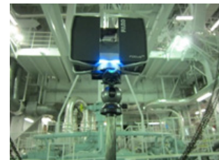
3D scanning systems provide highly accurate 3D representations of complex shipboard spaces that can be utilized for modernization and repair planning.
