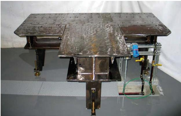
Newly Designed Large Diameter Pipe Shop Work Bench with Services (Gas, Power, Compressed Air) Routed via Covered Trenches
