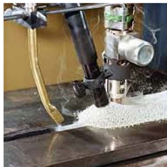
Submerged Arc Welding In Process
