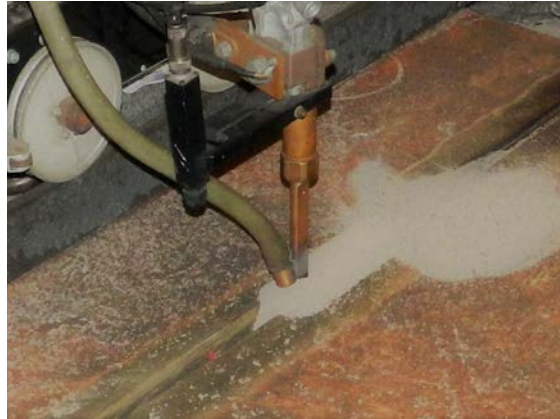
Submerged Welding Process (courtesy HII-NNS)
